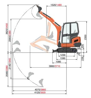
1190 mm arm/1810 mm boom 1090 mm arm/1690 mm boom Unit: mm
